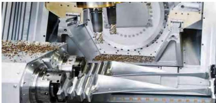
The modular IndraMotion MTX system controls standard and universal machines for milling, turning, drilling, grinding, nibbling, punching, shape cutting, and bending easily, quickly, and effectively. Proven CNC functions cover a broad range of applications from highly precise and quick machining of free-form surfaces to the most-demanding grinding applications, as well as plasma, laser, or waterjet machines.
